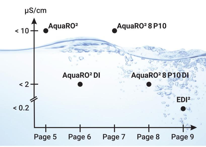
The series of AquaRO<sup>2</sup>, AquaRO<sup>2</sup>DI and EDI<sup>2</sup> are based on a reverse osmosis (RO) unit to produce deionised water. The EDI<sup>2</sup> series further processes the osmosis water by using an EDI cell to get type II water.
